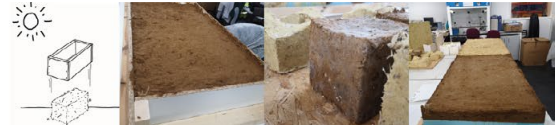
Step 5 : Let it dry. After filling up the mold up to the level needed, leave it to dry for 3 days. Afterward, gently remove the mold from the mixture to let it dry faster.
