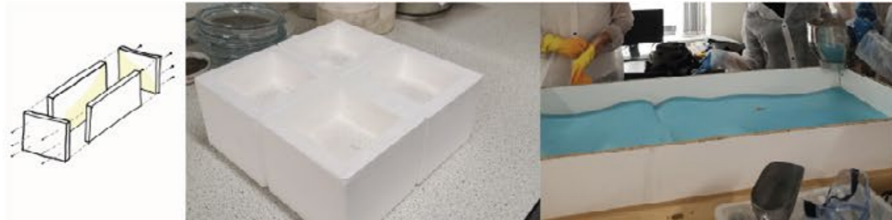
Step 1 : Make the mold. We use recycled wood to make the mold. The size of the mold depends on the size of the panel needed. Cover the inside surface of the mold with oil.
