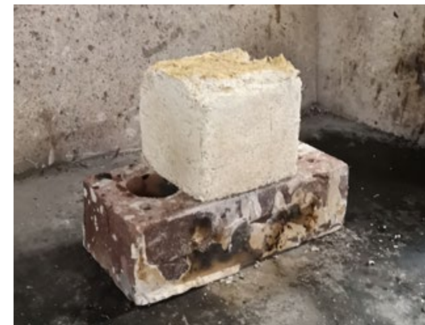
iii. Prototype 3 Date of created : 15th June 2021 Water, Lime & Bagasse Ratio : 1:1:4
