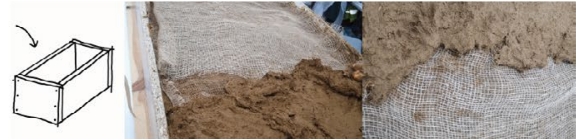
Step 4 : Pour mixture into the mold. After the mixture is mixed thoroughly, pour the mixture into the mold. Evenly spread the mixture into the mold.
