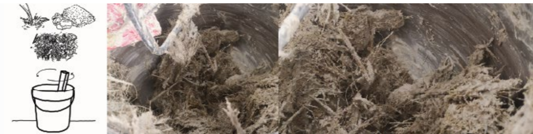
Step 3 : Mixture. Mix the material thoroughly. Do mix the lime and water first, then add bagasse bit by bit. Let it mix for 1 minute or more.
