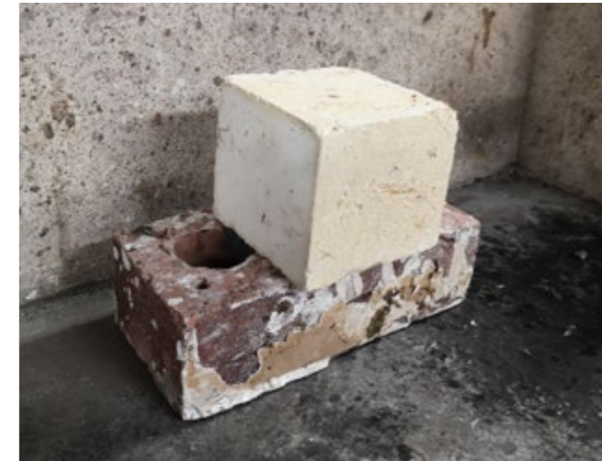
i. Prototype 1 Date of created : 10th June 2021 Water, Lime & Bagasse Ratio : 1:2:2
