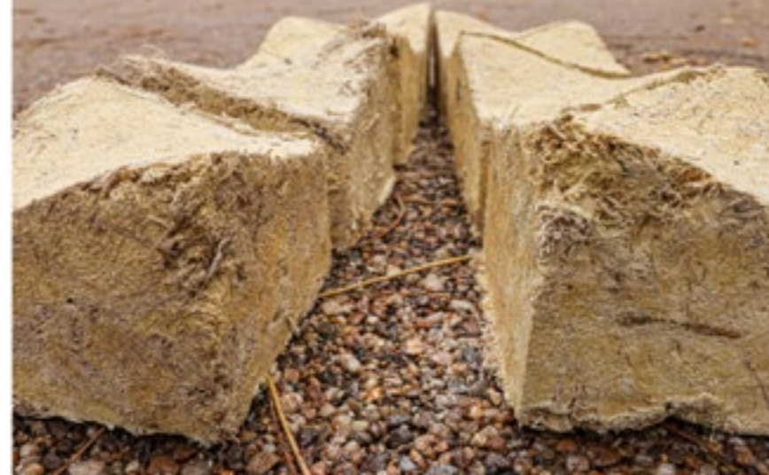
Prototypes 12 and 13 - Horizontal Patern - 325L / 650W / 80B
