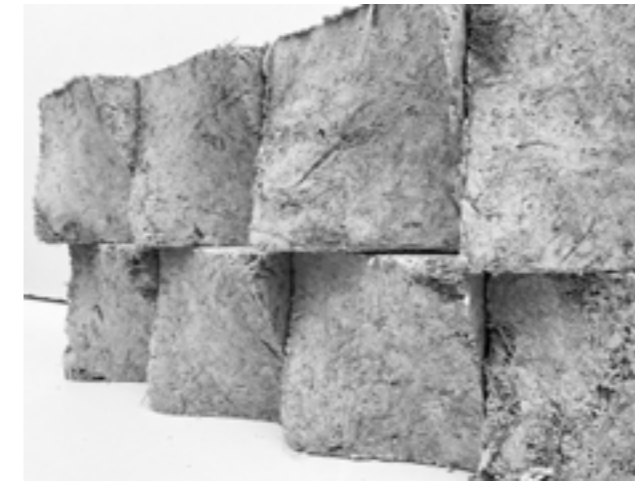
Fig.02 - Bagasse & Quicklime bricks
