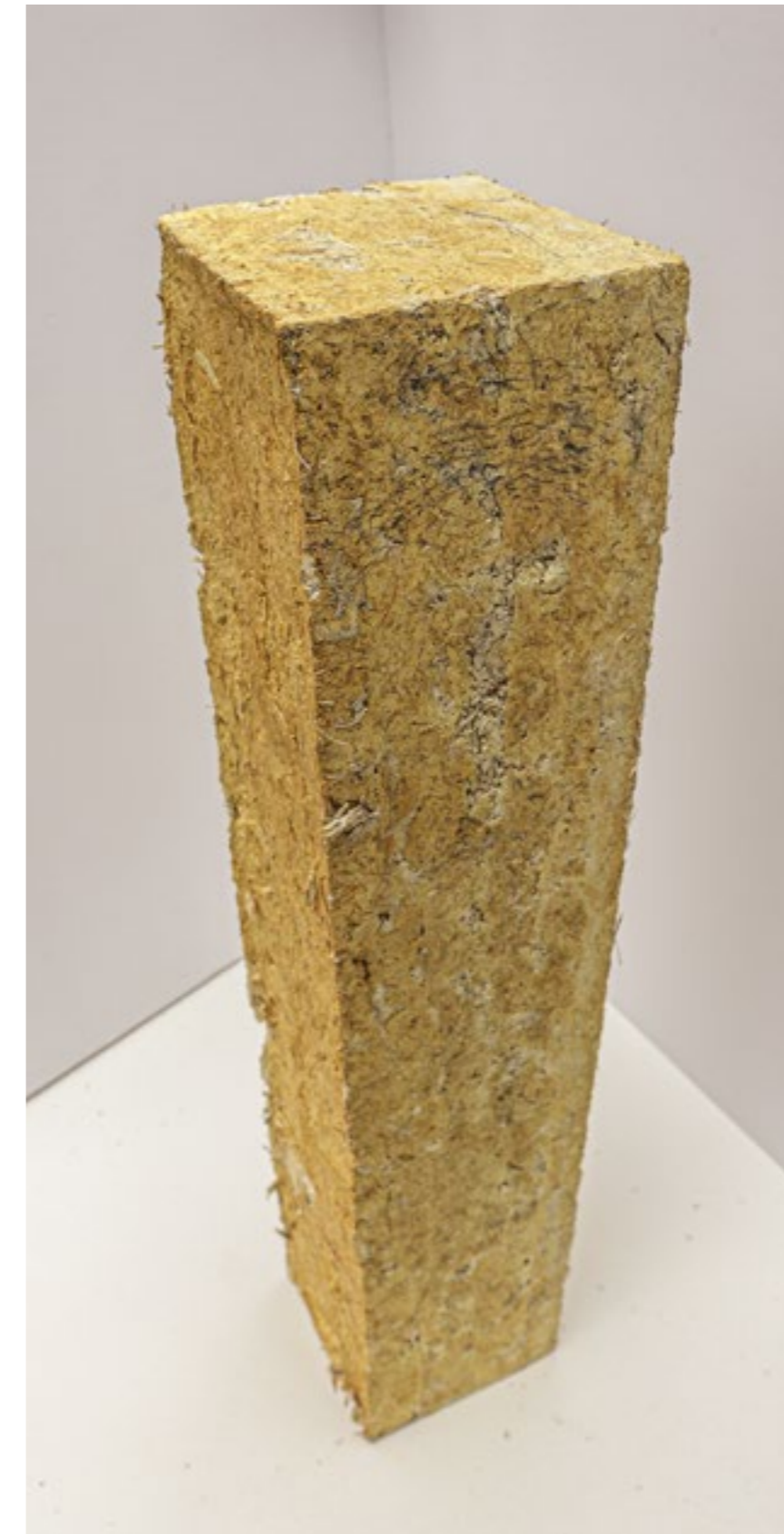
Prototype 14 - Structural Beam - 325L / 675W / 80B
