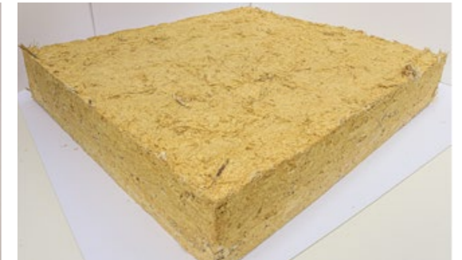
Prototype 9 - Thermal Insulation Board - 325L / 675W / 80B
