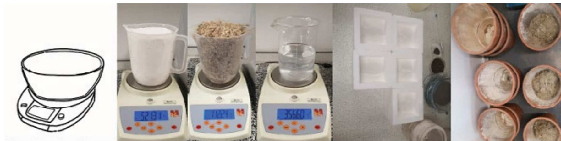
Step 2 : Weight and prepare the material. Weight and prepare the materials of water, lime & bagasse.
