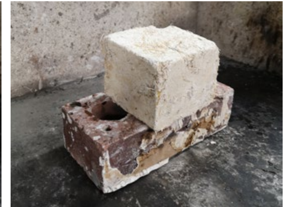
ii. Prototype 2 Date of created : 10th June 2021 Water, Lime & Bagasse Ratio : 1:2:3
