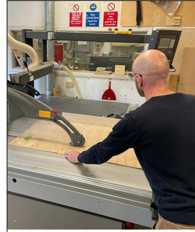
Fig. 46 - CUTTING THE WALLS
