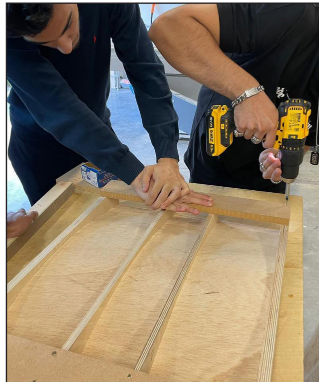
Fig. 56 - SCREWING THE REINFORCEMENT SYSTEM
