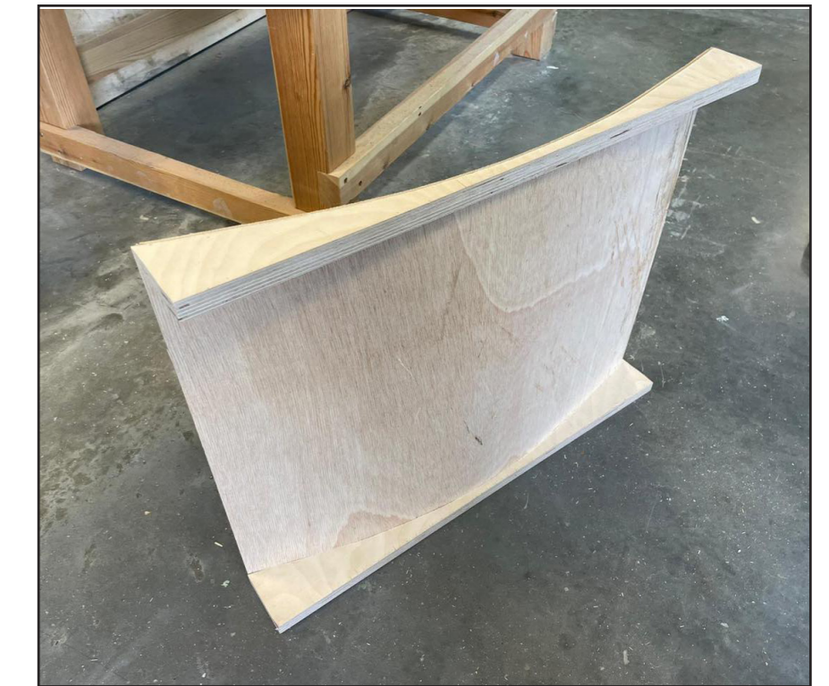
Fig.54 - BACK VIEW OF THE LARGE CURVE SHOWING THE TOP AND BOTTOM RIBS
