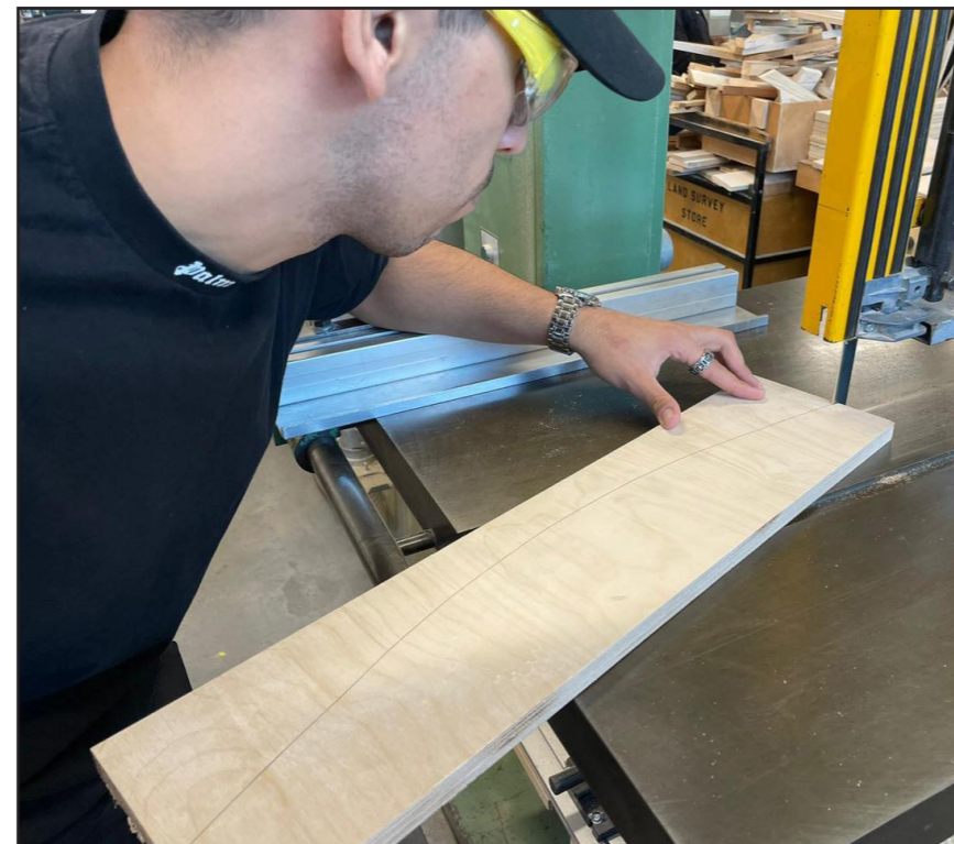
Fig.51 - CUTTING THE RIB
