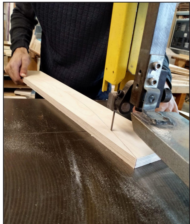
Fig. 50 - CUTTING THE RIB
