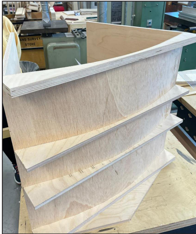
Fig. 55 - BACK VIEW OF THE FOUR RIBS MAKING THE CURVE
