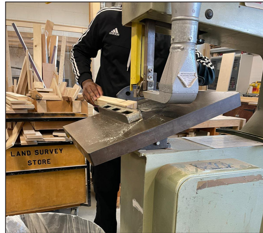
Fig. 63 - CUTTING THE BATTENS AT AN ANGLE
